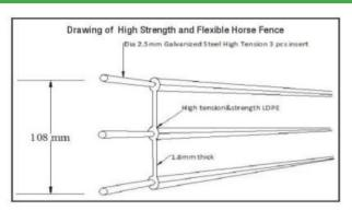
Watt Plastics Flexible Stud Rail is 108mm wide and contains 3 steel wires for extra strength . The rail attaches at end posts and slips freely through the line post brackets to allow rail flexibility. We recommend post spacings between 3 and 4m and we do not recommend straining more than 100 per run.
